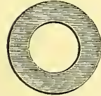
Rings for water bath, for adapting the bath to hold any size basin. § 118.
